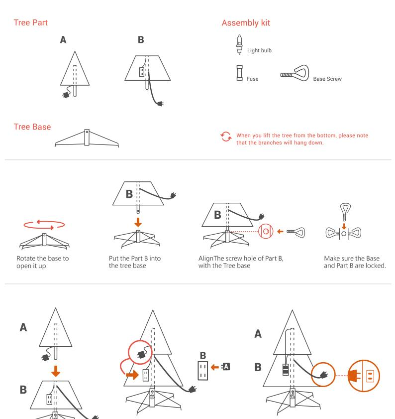
Connect the plugs on the Parts A to the socket on the part B.
